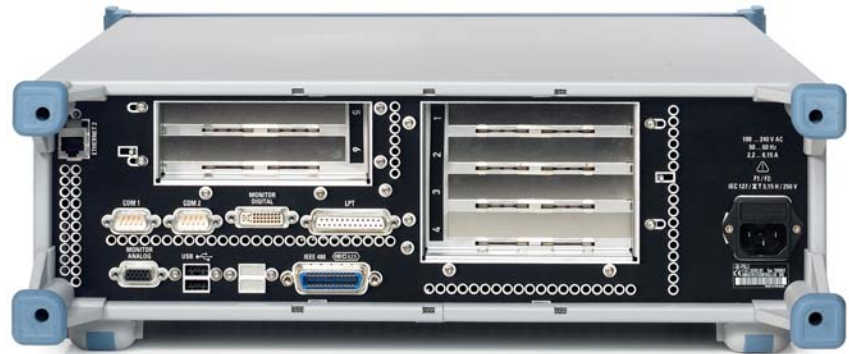
Rear view of the PSL3: View on the interfaces and free PCI and ISA slots
